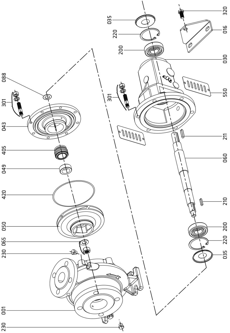
**Bearing Bracket with Oil Lubrication**
