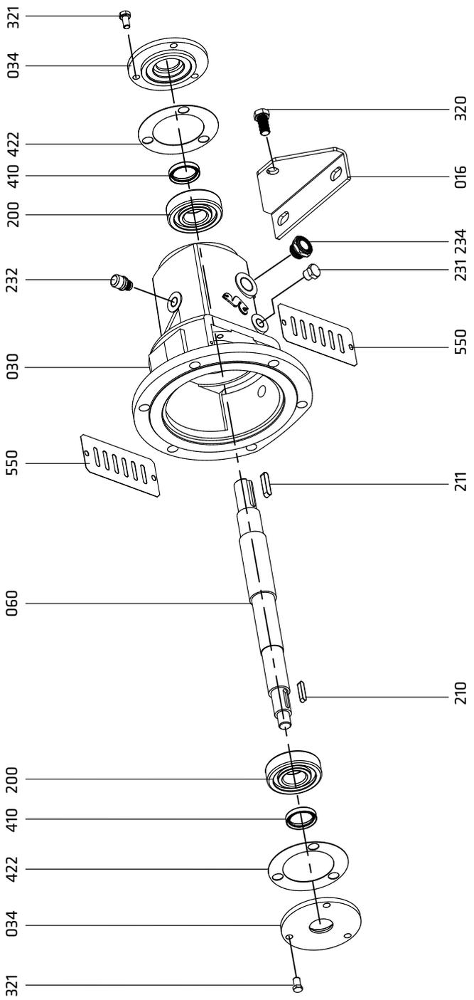
**Bearing Bracket with Grease Lubrication**
