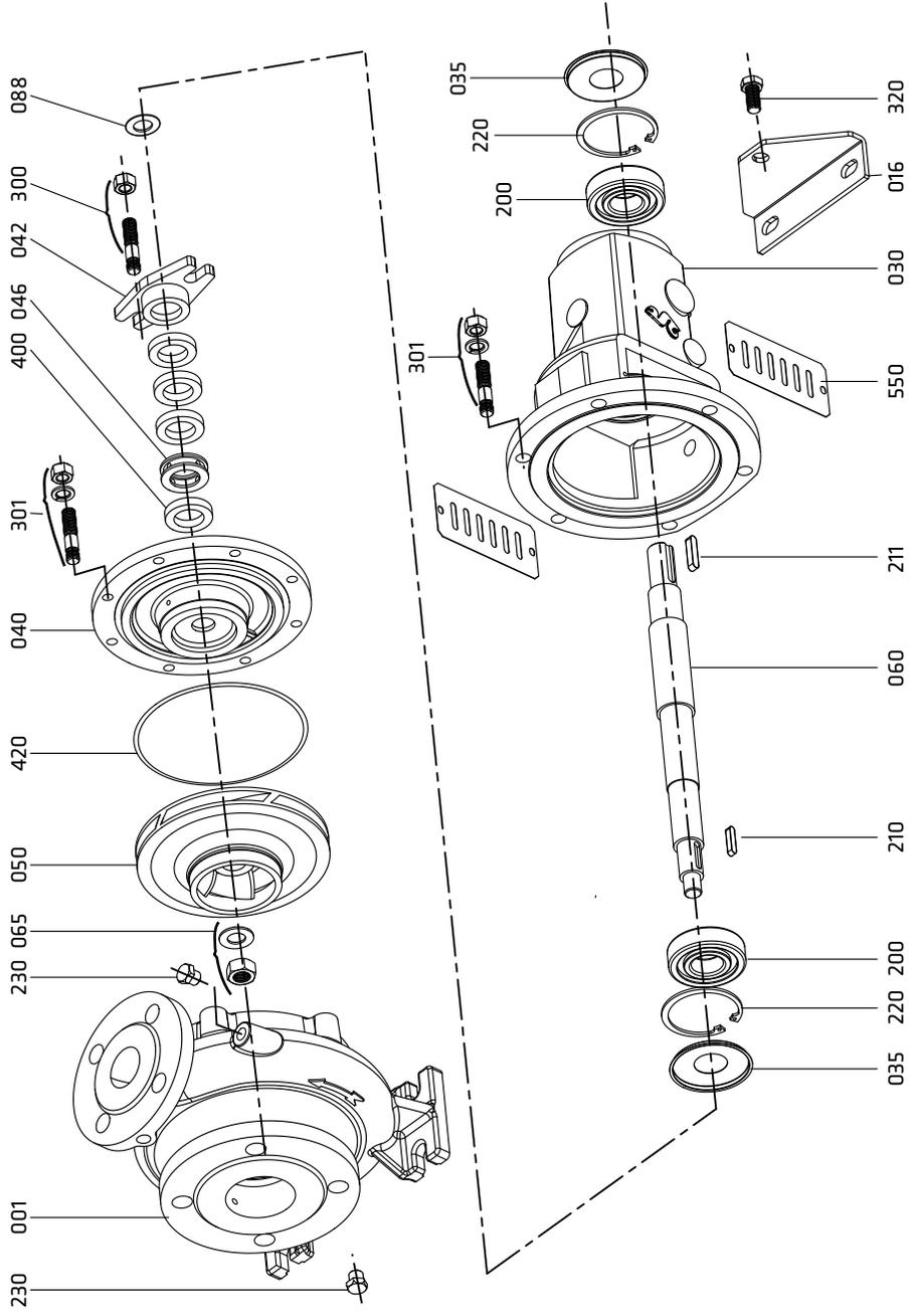
**Form: F1 (Pump with Mechanical Seal)**
