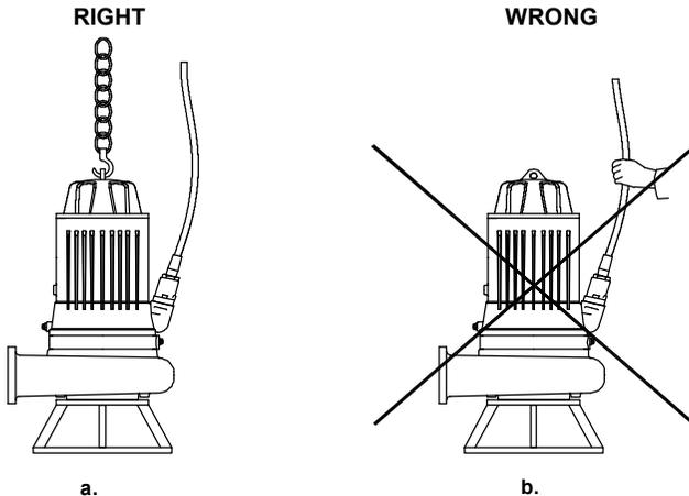
Figure 1. Lifting the pump property
