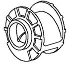
**D type impeller** : It is also closed type, suitable for high speed motors (2900 or 3500 RPM). It is convenient for high pressure, small capacity and smaller size solid particles.
