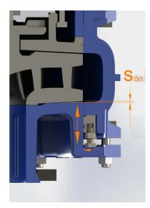
SSP-V series HC model pumps have front gap adjustment. Stop bolts in front of volute casing can set the gap between inlet port and impeller. Therefore negative effects of wearing optimise and servise time of the pump improes. Besides that there is no need diassembly of volute casing and time is saved accrodingly.
