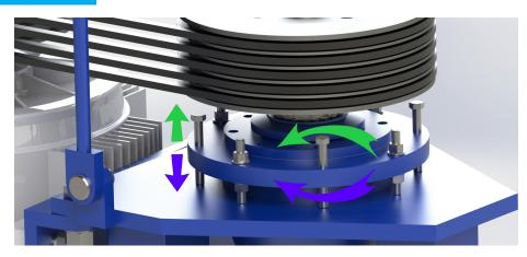
SSP-V series pumps have ability to move back and front by tightening and loosening the studs on the cartridge bearing housing. In this way, the clearance between the impeller and the wear plate is controlled. Back-side clearance adjustment allows to keep the pump performance at the highest level even if pump abrasions occur.
